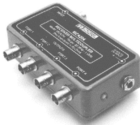
Models MC102, 104, 202 and 204 are passive couplers, and therefore need no external power to operate. However, because of the passive design each coupler will exhibit some signal loss from input to output ports. A 2-port device has slightly more than 3 DB signal loss, and a 4-port slightly more than 6 DB loss. On a receiver with a calibrated S-meter this will result in a reduction of meter reading of 1/2 S-unit for a 2 port coupler and about one S-unit for a 4-port coupler.
